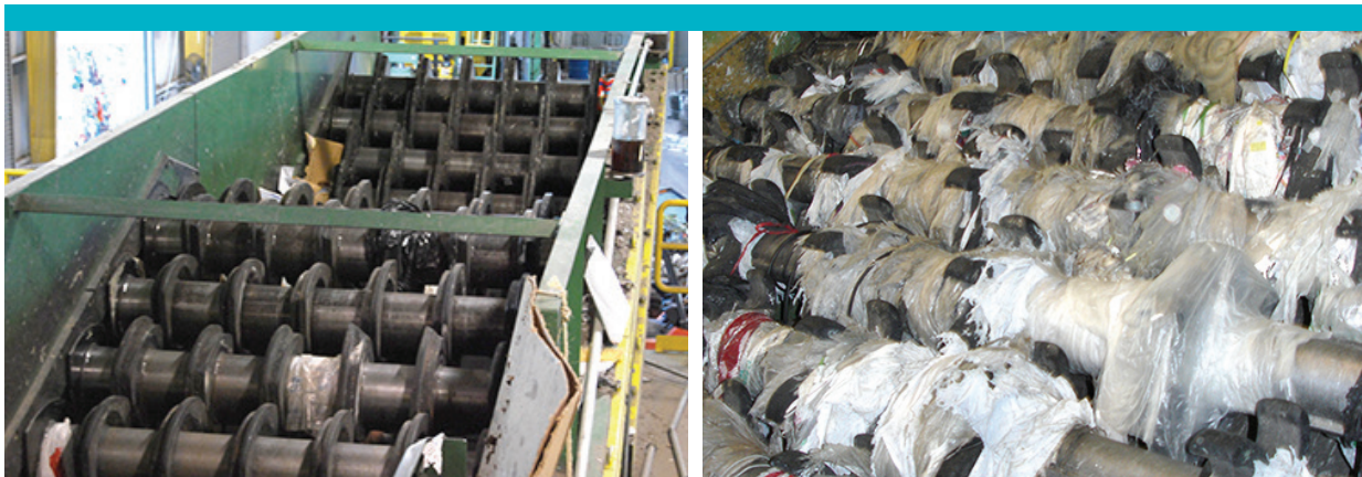
Thin films are one of the biggest challenges for MRFs because these materials get tangled around the sorting equipment, costing recycling facilities thousands of dollars per year in maintenance costs. Above: Before and after photos of sorting equipment with tangled plastic bags and films.
